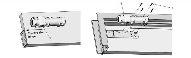
NOTE: Orient pinion (1) closest to hinge.
